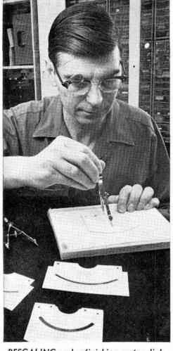
RESCALING and refinishing meter dials is one of the jobs carried out by Kent Johnson.
